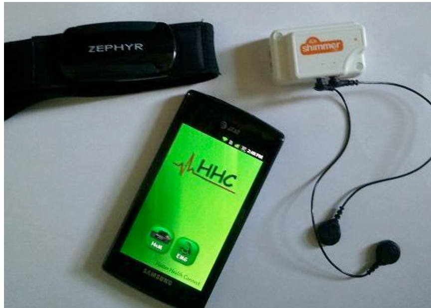
Figure 3: The Zephyr HxM Monitor (left), Intel Shimmer (right), and Samsung Captivate (bottom)
