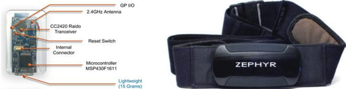
Figure 3(a): The Intel Shimmer internals, Figure 3(b): the HxM heart monitor
